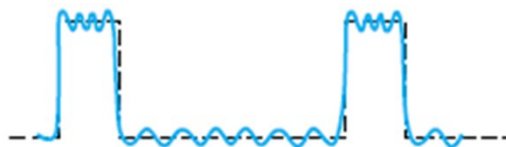
Figure 3.8 Effect of Bandwidth on a Digital Signal
