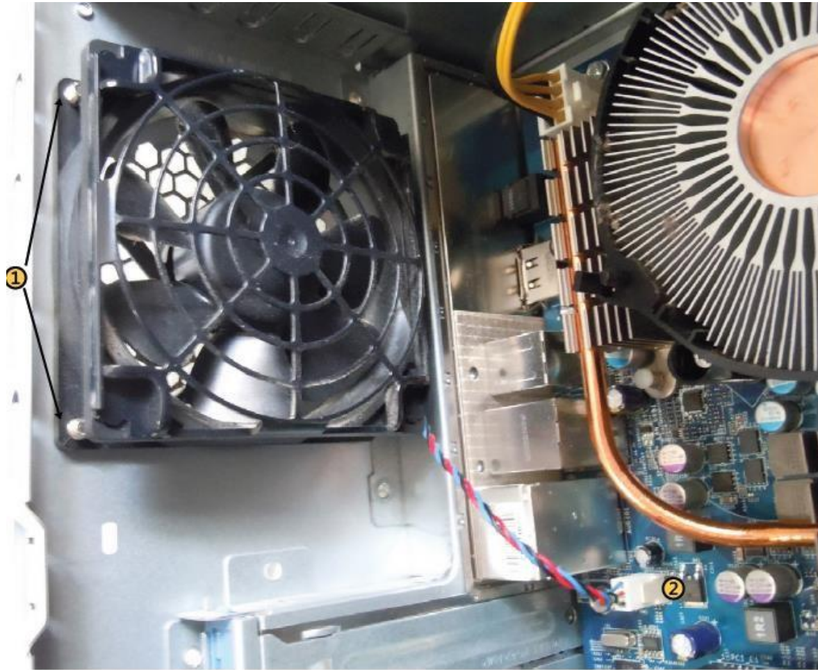
FIGURE 1-3 Removing a case fan
