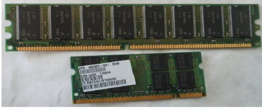
FIGURE 3-2 Comparing a DIMM and a SODIMM.
