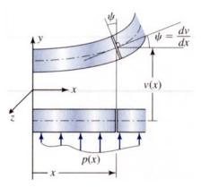
• The deflected curve represented by v(x) is called the Elastic Curve.
