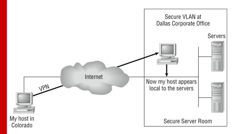
A VPN actually makes your local host part of the remote network by using the WAN link that connects you to the remote LAN. The VPN will make your host appear as though it's actually local on the remote network!
