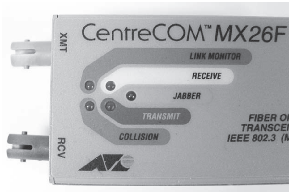
FIGURE 5.5 A 100Base-TX to 100Base-FX transceiver
