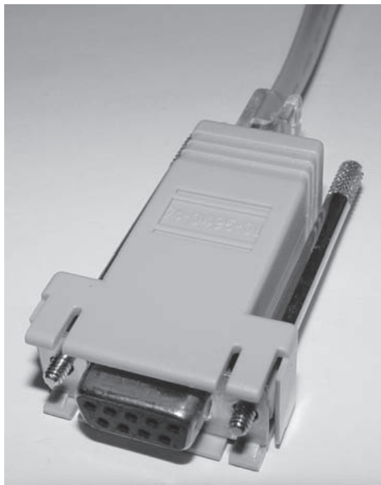
FIGURE 3.9 An RS-232 cable end
