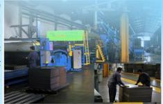
The production capacity of this company is in the field of producing geomembrane sheets and single sheets up to 2 meters in width.
